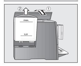
Open the lid on the left hand side of the coffee system ①. Pull the water tank up and out using the handle ②. ■ Fill the water tank with fresh, cold tap water to the "Max." mark.
